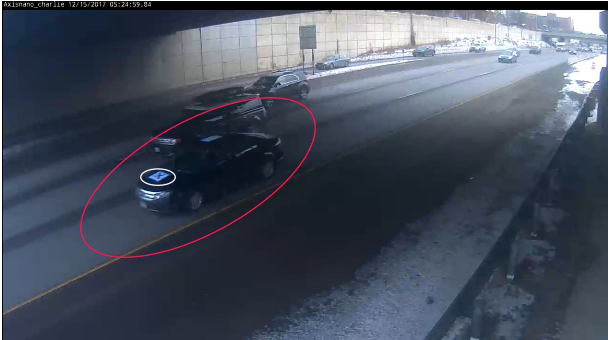
Figure 4.1 Test vehicle. Note the markings on the front, top, and rear of vehicle for identification.
