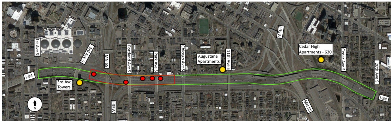
Figure 2.1 Original Testbed site showing radar sites (red dots), radar coverage (outlined in red), rooftop stations (yellow dots) and camera coverage (outlined in green).
