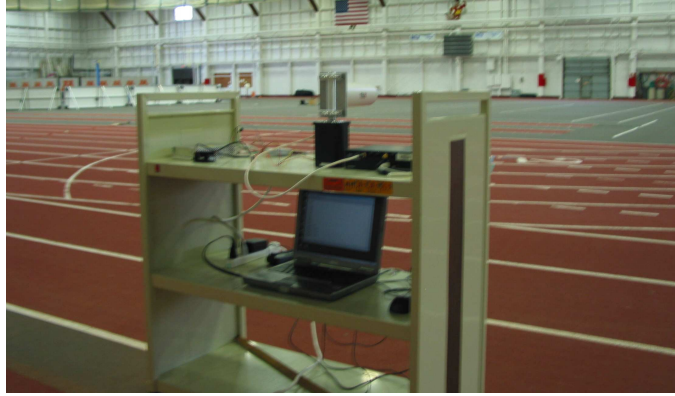
Figure 5.5: Experimental Setup: The reference node equipped with directional antenna.
