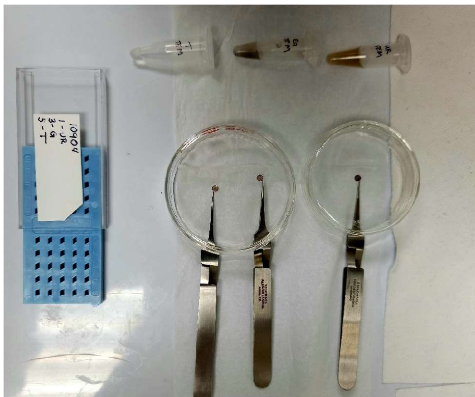
Figure A.5: TEM sample preparation drop casting samples onto grids and drying.
