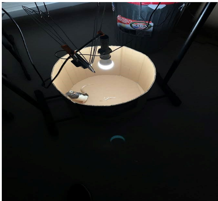
Figure 1: Early Prototype of the Open Field chamber. A cylinder constructed with cardboard and duct tape. A light source and camera are suspended from a coat rack and a rat is inside the chamber for preliminary testing. Testing was also conducted in the Behavioral Room to minimize environmental noise sources during recording.
