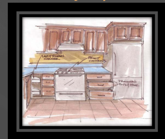
Accessible kitchen storage
