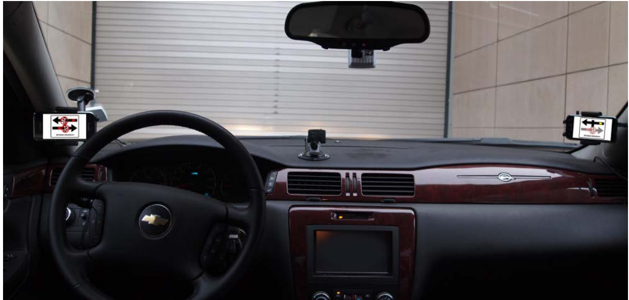
Figure 40. The location of the displays for the in-vehicle CICAS-SSA in the Field Study.
