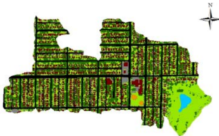
Figure 4.1 Original and modified land cover in GCP watershed. TIA increased from 34% to 44% in this watershed due to the un-shading process.
