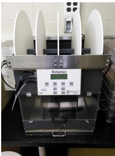
Figure 3. Rotamex Machine for Assessing Rotarod Performance. Four mice, one in each section, were placed on the Rotamex in each test.
