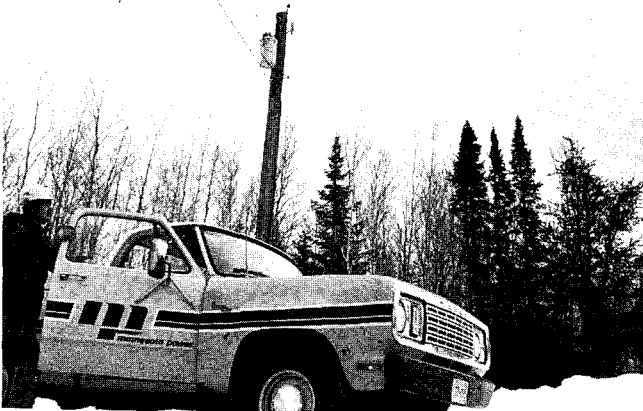
Overhead electric wires can be particularly hazardous on a landing. Call the power company if wires need to be raised.
