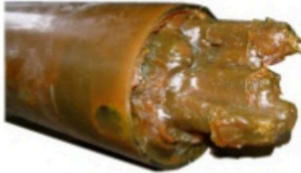
Figure 2.6 Tendon injected with wax
