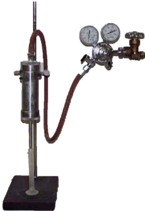
Figure 2.9 Schupack Pressure Bleed test apparatus [53]
