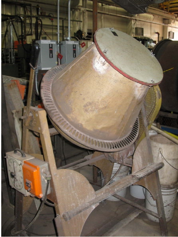
Figure 1 Sinter Cement Mixer – Dry Mixing
