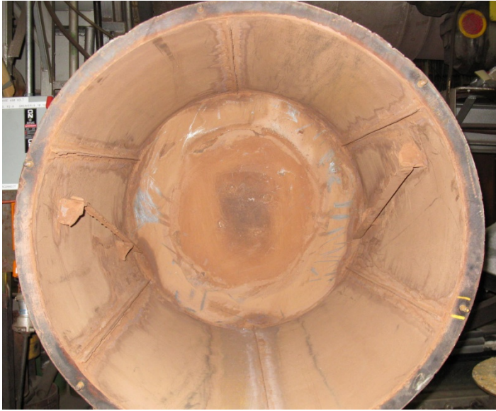
Figure 5 Sinter Granulation Drum Lifter Detail
