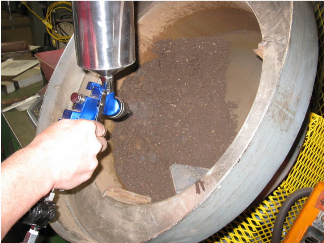
Figure 9 Balling Disc with Load and Water Spray Addition
