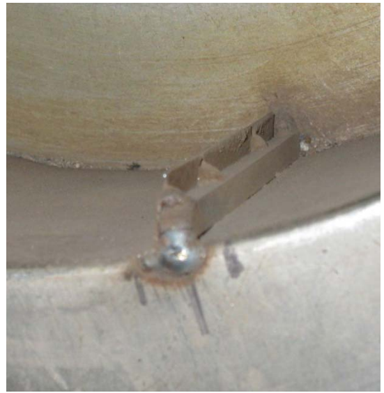
Figure 6 Balling Disc Lifter Detail
