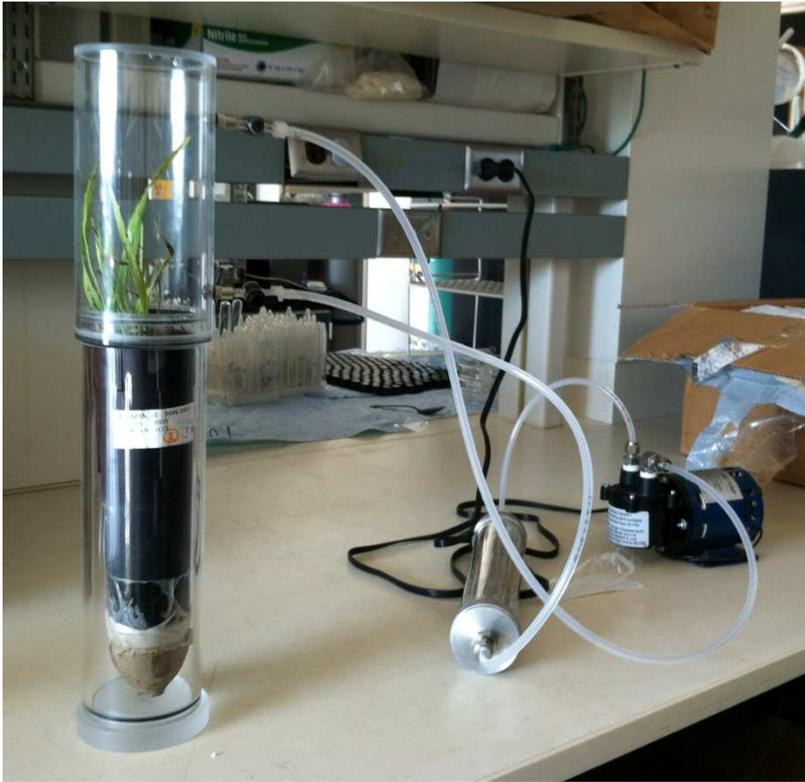
**Figure S3.1.** Whole-plant chamber used for CO<sub>2</sub> analysis.
