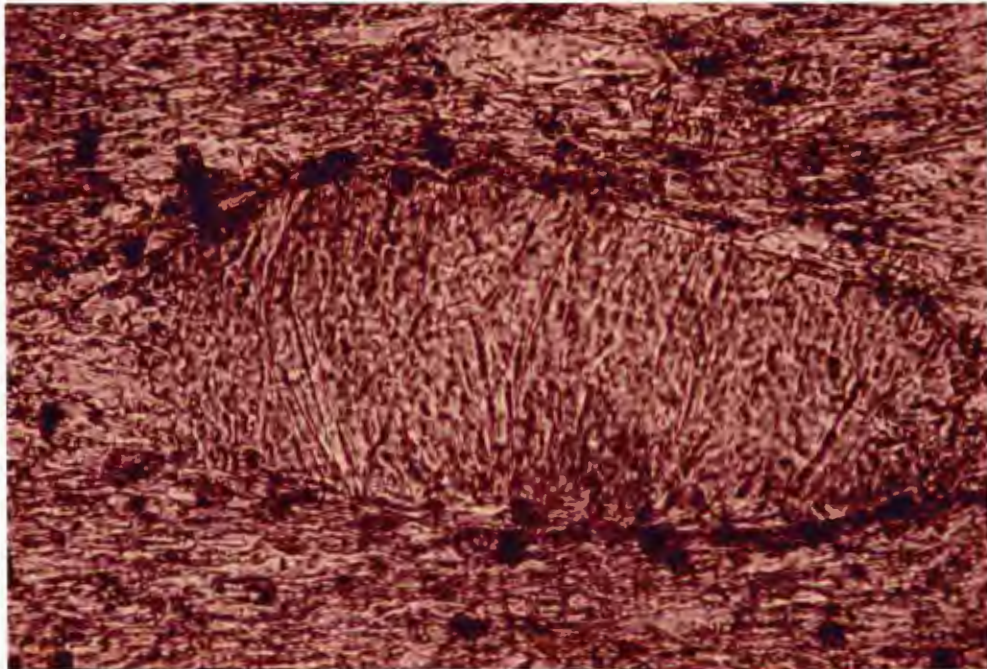
Fig. 38 Photomicrograph of a 'cross-mica' chlorite porphyroblast in slate. Note the elongation of the porphyroblast parallel to rock cleavage, the orientation of the mineral cleavage perpendicular to the rock cleavage and the strain shadows at the ends of the porphyroblast. 0.8 km SSE of Carlton. Field of view is 0.24mm X 0.17mm. Plain light.
