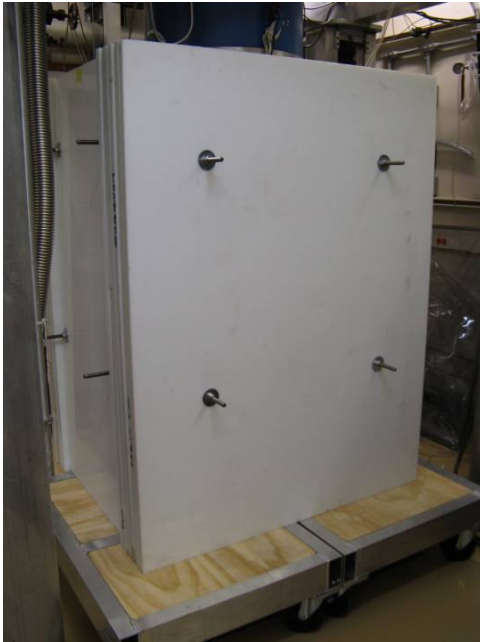
Figure 3.10: Final assemblage of the neutron shield around the dilution refrigerator.
