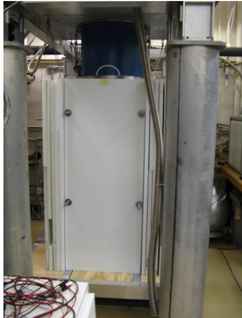
Figure 3.10: Final assemblage of the neutron shield around the dilution refrigerator.
