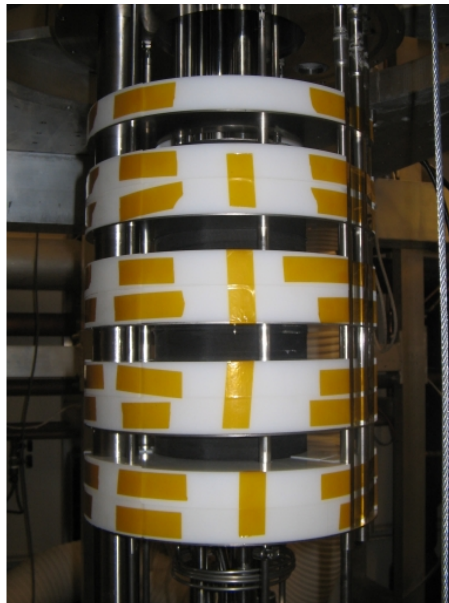
Figure 3.8: A picture of the baffle poly installed. The yellow strips are Kapton tape used to secure the pieces of poly together.
