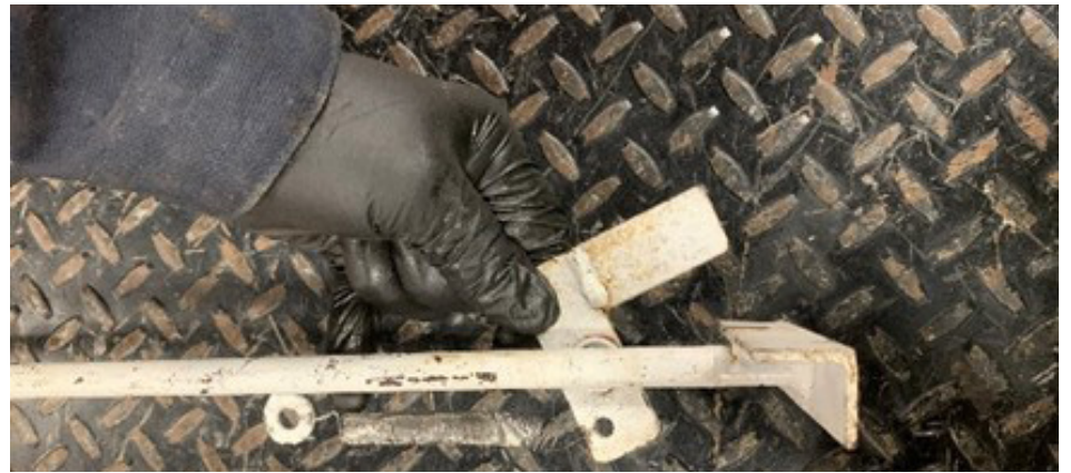
The chip-seal marker installation tool speeds up the process.
