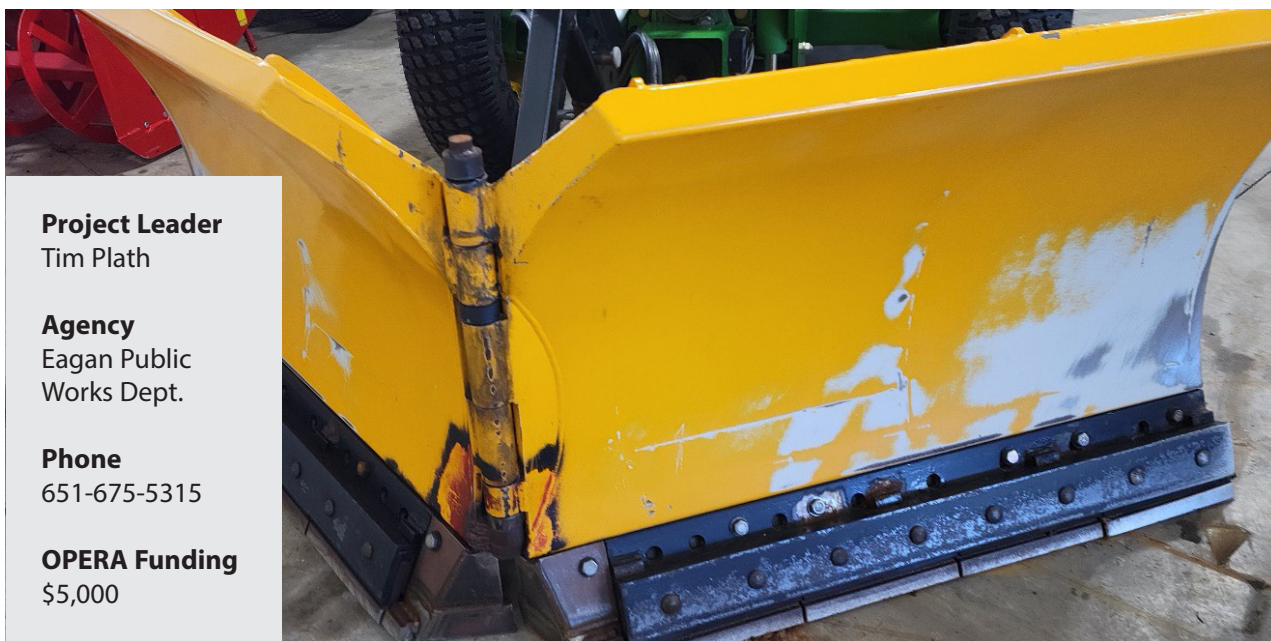
The project team used segmented and flexible tungsten carbide plow cutting edges.
