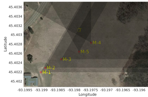
Fig. 9 A sample field experiment at Cedar Creek Ecosystem Science Reserve, MN. The target location is marked by “T”. Each measurement is shown as a gray wedge. The UAV starts at the first measurement location M1. Until the fourth measurement, the UAV applied the doubling strategy. After that, the halving strategy was applied. After the fifth measurement, the target was localized to the desired localization uncertainty. The dark gray area is the resulting intersection of all the measurements, showing the area where the target is.
