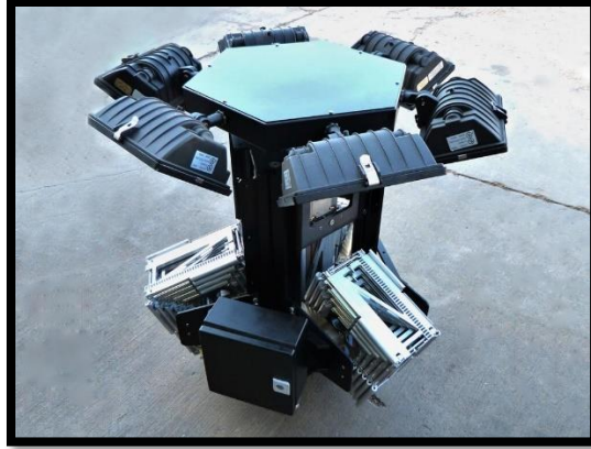
Figure 13: Tower solutions linear actuator equipped with flood-light apparatus
