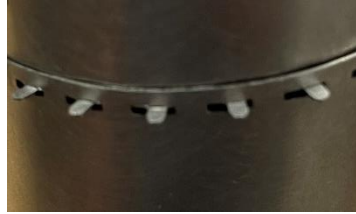
Fig 3: Close up view of the tab-slot engagement
