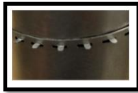
Figure 28: Close up showing tab and slot engagement
