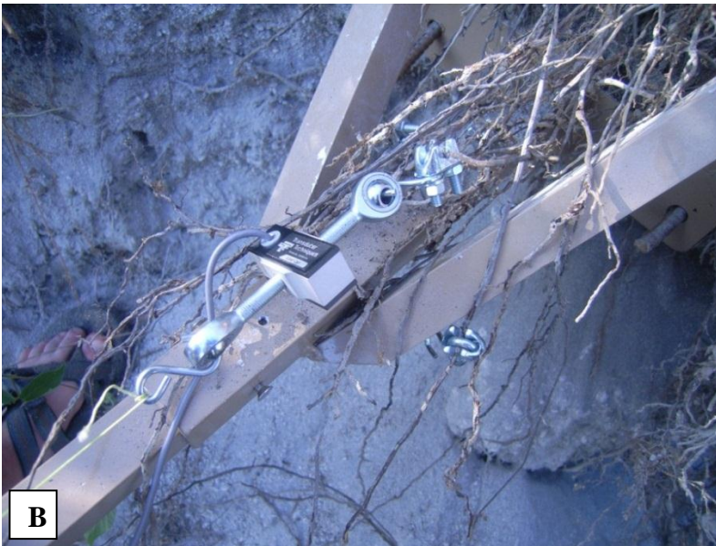
Figure 4-2. Root tensile strength and stress displacements were measured using a device called a Root-Puller. This device was composed of a metal frame with a winch attached to a load cell and displacement transducer and a data logger. Different size roots were attached to the load cell and displacement transducer using u bolts of various sizes. The winch was then cranked at steady rate until the roots broke. Only roots belonging to Saccharum spontaneum , the dominant grass at both field sites, were tested.
