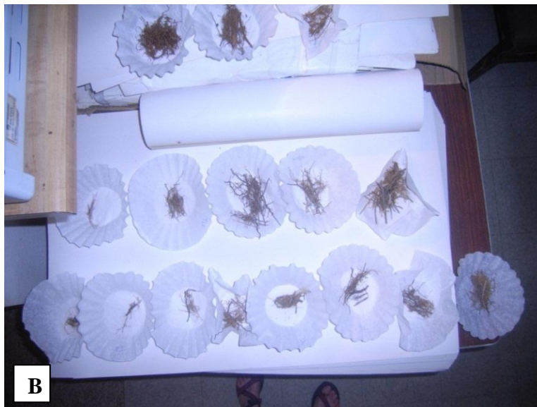
Figure 4-3. Root density data were collected on various sizes of Saccharum spontaneum and Parasponia rugosa . These data were used in obtaining values for the added cohesion to the soil matrix provided by root networks. (A) A single stem of Saccharum spontaneum , an example of a stem that was tested for root.
