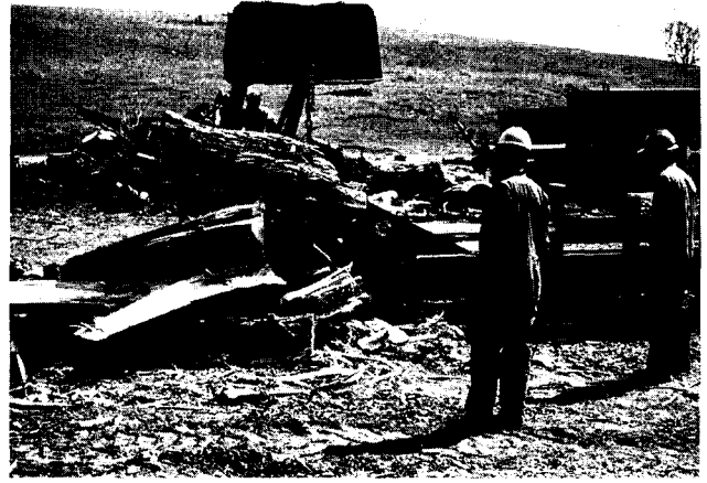
Figure 3: Material of larger diameter must be split before being passed through the Metro-chiparvester, a machine designed for chipping whole trees. The splitting process also helps to locate hidden metal objects.
