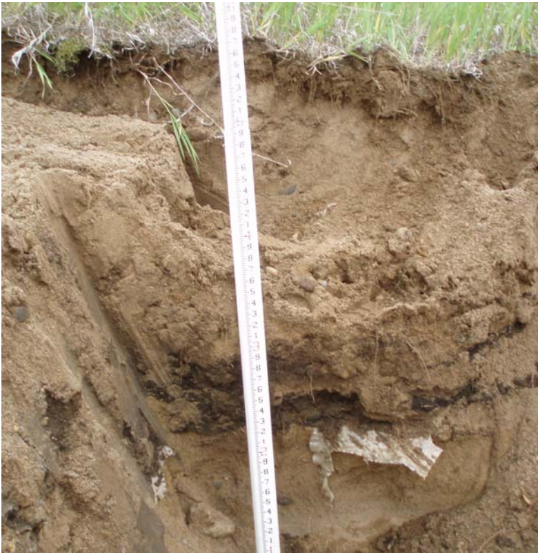
Photo 6 Former Lagoon Liner at SOC3-TT2
