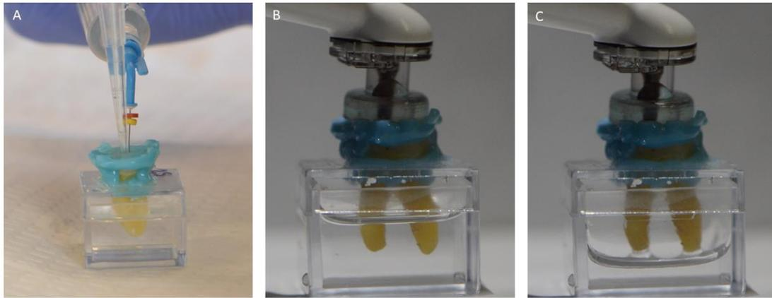
Figure 6: Irrigation apparatuses. Panel A displays irrigation and suction for reads #1, 2, 4, and 5. Panel B shows a molar and liquid in an acrylic box before GWS irrigation and Panel C displays the apparatus after GWS irrigation with remaining solution at the level of the apices of the molar.
