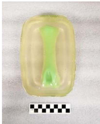
Figure 2. A medical gelatin block with an inserted dog chew toy bone.
