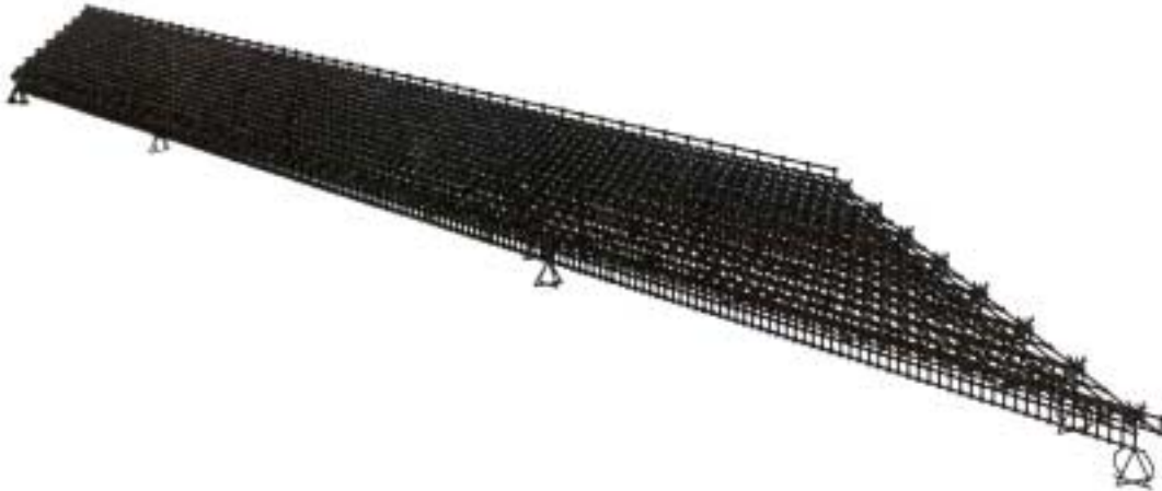
Figure 3.1 Finite Element Model of Mn/DOT Bridge No. 27734
