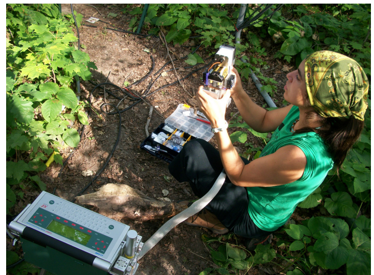
Field technician fixing LI-COR machine for measuring respiration rate in plants. July 2011.
