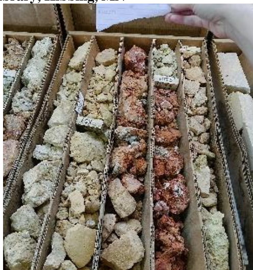
Figure 13. Drill core from the Thistledew Lake Sequence.
