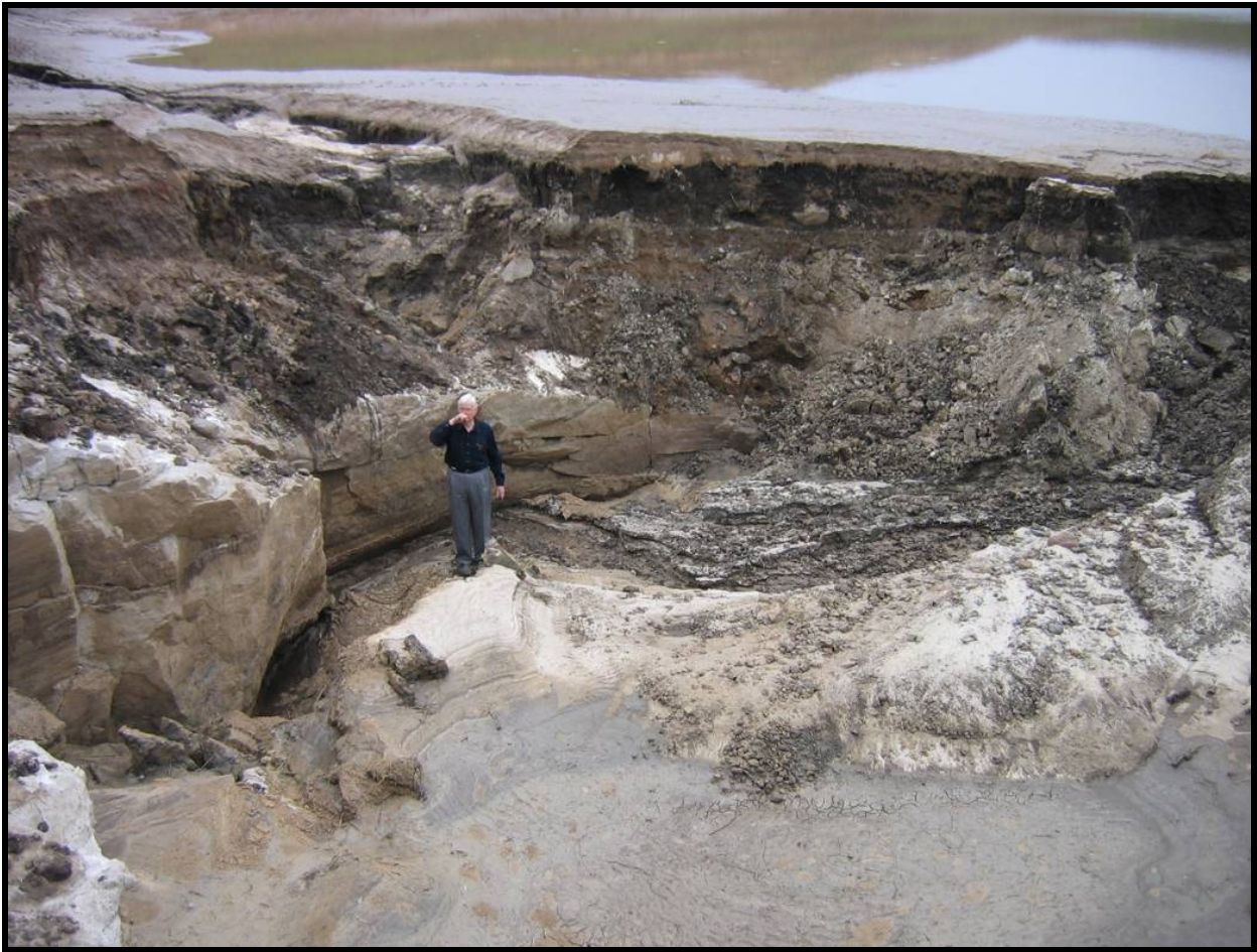
Figure 7. Close up photo of the largest sinkhole that drained the Dancing Waters storm water retention pond
