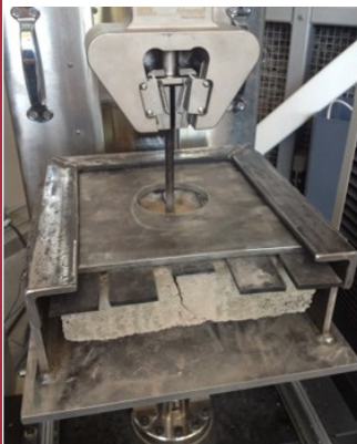
Left: Bond pull-out tests that were conducted during the rapid set patching materials project Above: finite element model of the test
