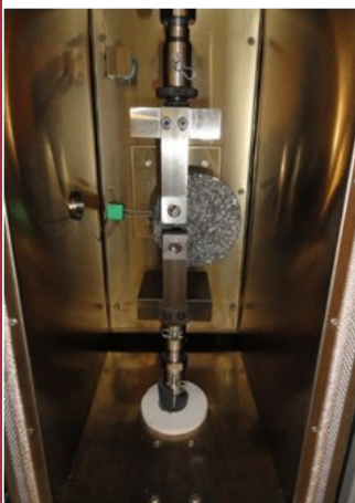
Left: The disk-shaped compact tension (DCT) test for determining thermal cracking potential of asphalt mixes; Above: Thermally induced crack in North- Western Minnesota
