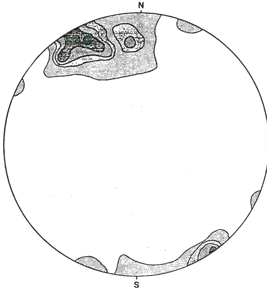
FIGURE 8 - STEREOGRAPHIC PROJECTION OF 78 POLES TO CLEAVAGE COUNTED ON A KALSBECK COUNTING NET AND CONTOURED AT 3, 8, 13, 18, AND 23 PERCENT OF TOTAL DATA PER 1 PERCENT AREA.
