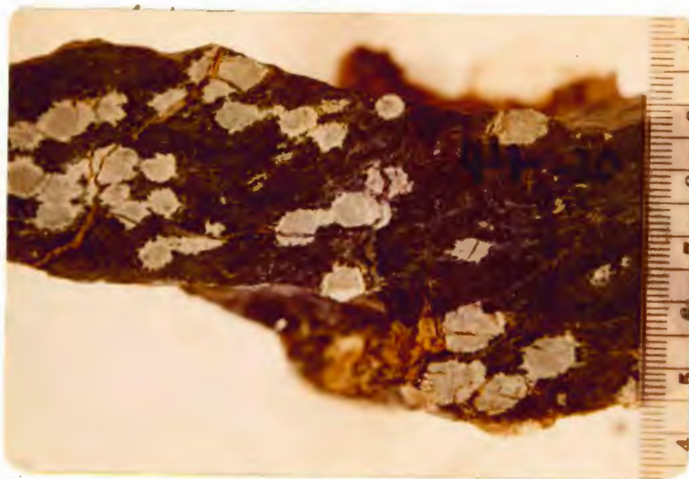
PLATE 8. Photograph of light green varioles in variolitic metabasalt. Sample from a localized thin horizon in more massive metabasalt flows. Scale in cm. Sample no. 44-20.
