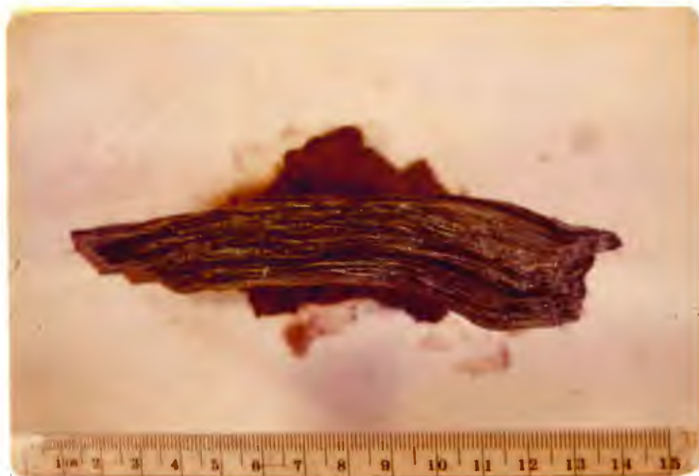
PLATE 6. Photograph of highly schistose metabasalt sample with crenulations in rock cleavage. Rock taken from fault zone. Scale in cm. Sample no. 10-3.
