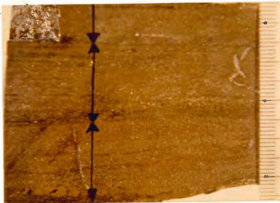
PLATE 33. Photograph of massive sulfide rock composed of pyrite and silica. Two beds and part of a third with graded bedding (Top to Top of Photo) are indicated. Scale in cm. Sample no. MNER-213.
