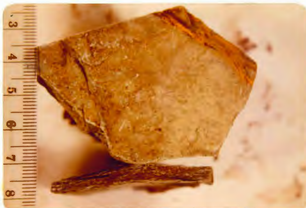
PLATE 13. Photograph of muscovite phyllite sample. Note slight crenulations in schistosity, pale grey-green micaceous appearance, and iron oxides after pyrite along foliation planes. Scale is in cm. Sample no. 52-8.
