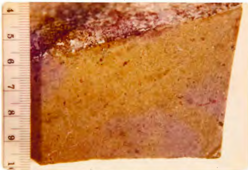
PLATE 30. Photograph of altered basalt from outer zone of contact metasomatic aureole around granodiorite stock. Fine-grained to microcrystalline buff colored alteration assemblage is well developed. Scale in cm. Sample no. 16-9S.
