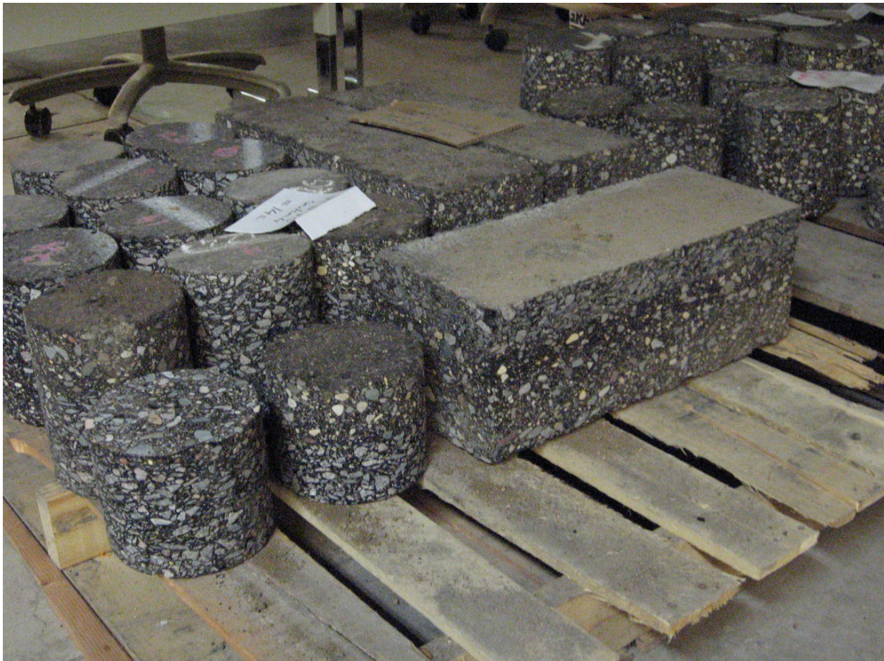
Figure 6. Asphalt pavement specimens at the University of Minnesota's Department of Civil Engineering.
