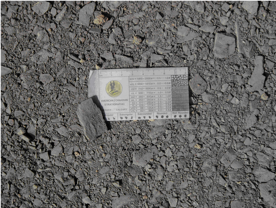
FIGURE 7 Mesabi Hard Rock™ Class 5 used on 6th Ave. in Virginia, 2006. Photo by M. Meinders Patelke.
