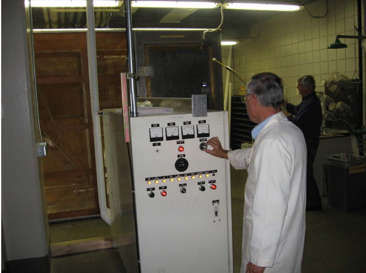
Figure 8. Successful operation and leakage monitoring of 15kW microwave unit and test chamber (in the foreground is David Lindroth, and in the background is David Hopstock, Ph.D., of David M. Hopstock and Associates, LLC).
