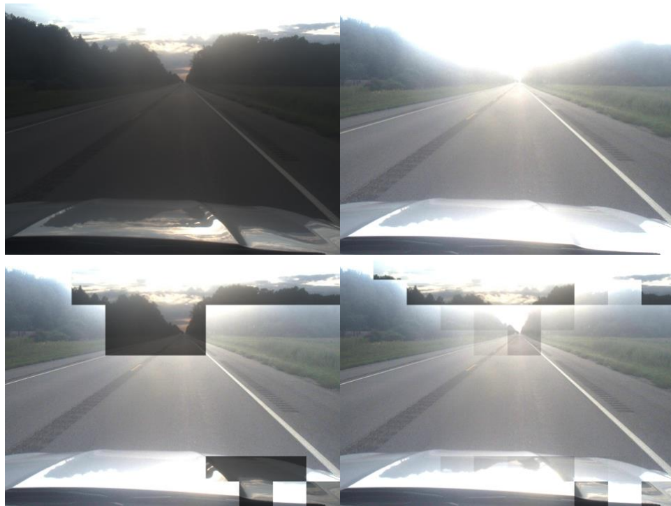
Figure 4.10: Source image (left-top), DCI (right-top), L-DCI (left-bottom), VL-DCI (right-bottom)
