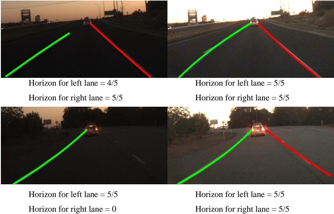
Figure 3.12: Quantification of detections by LaneNet on source dataset (left), contrast improved dataset (right)
