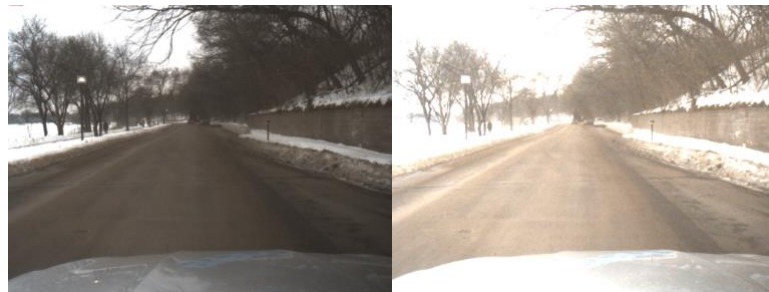
Figure 3.13: Issues with contrast improvement, source image (left), contrast improved image (right)
