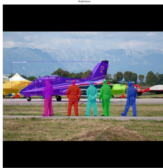
Figure 4.5: Segmentation output for MaskRCNN model
