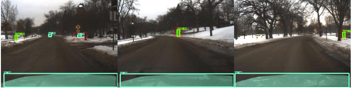
Figure 2.10: False positives for MaskRCNN shown in dashed rectangles
