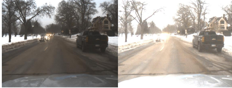
Figure 3.14: Issues with contrast improvement, source image (left), contrast improved image (right)
