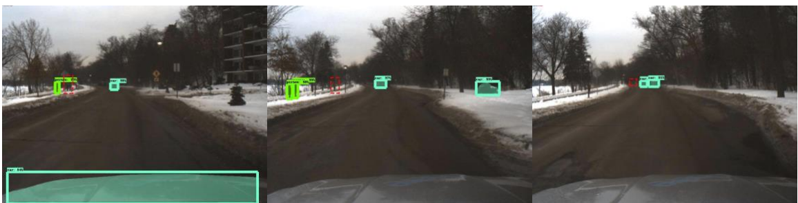
Figure 2.9: False negatives for MaskRCNN shown in dashed rectangles
