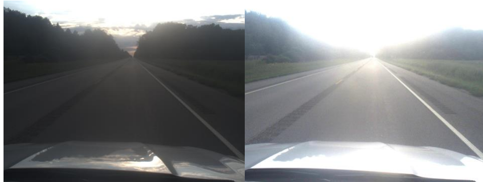
Figure 4.3: Source Image (left), Image after DCI implementation (right)
