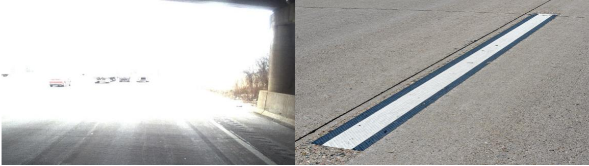
Figure 2.2: (a) Visual feed of vehicle exiting a tunnel, (b) A high contrast lane marking
