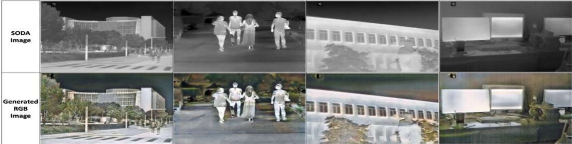
Figure 13: The first row shows samples of the original SODA-5 l . The second row shows their corresponding generated RGB images translated by CycleGAN.
