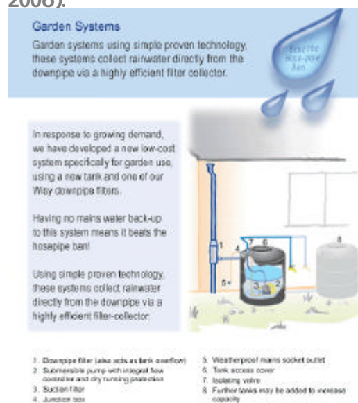
Figure 9. Diagram of a rain harvesting system that would be used in smaller facilities (rain harvesting systems 2006).
