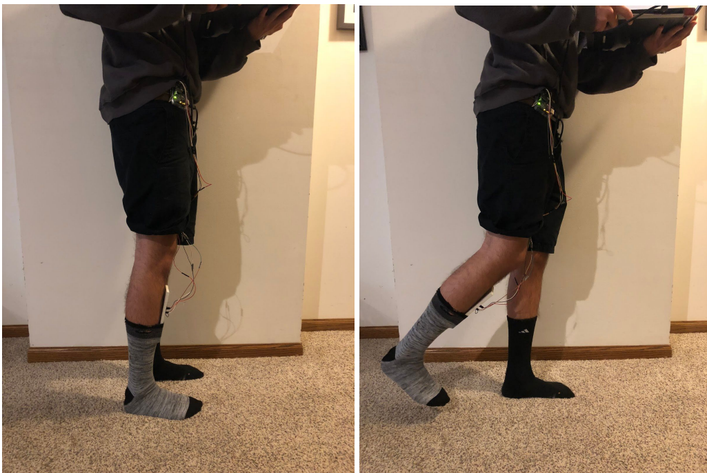
Fig. 11 Swinging monitored leg backwards to calibrate system.
