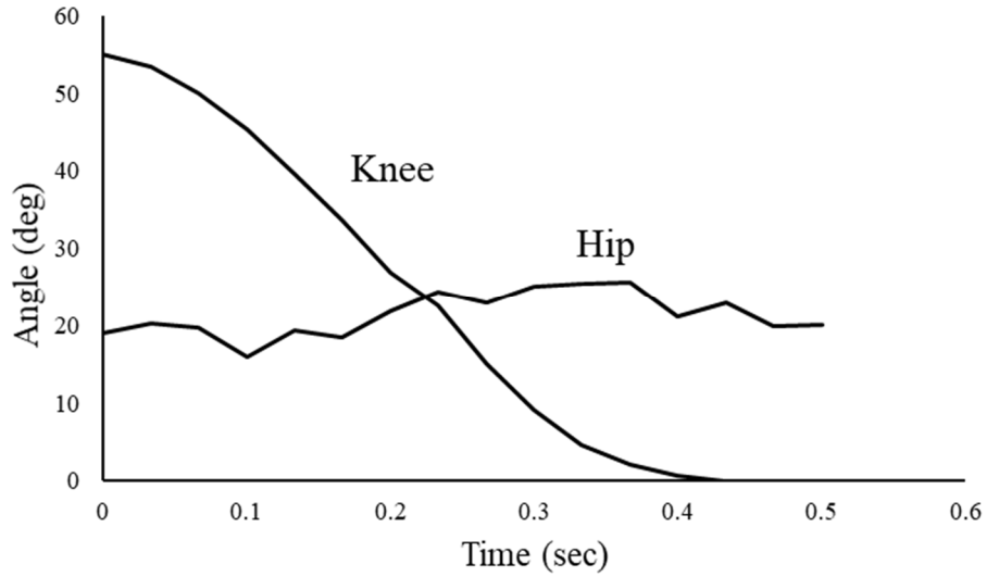
Figure 3.5: Knee and hip angles for the knee extension phase of gait. This phase took 0.5 sec, knee angle changed from 55 deg to 0 deg, and hip angle remained constant around 20 deg.
