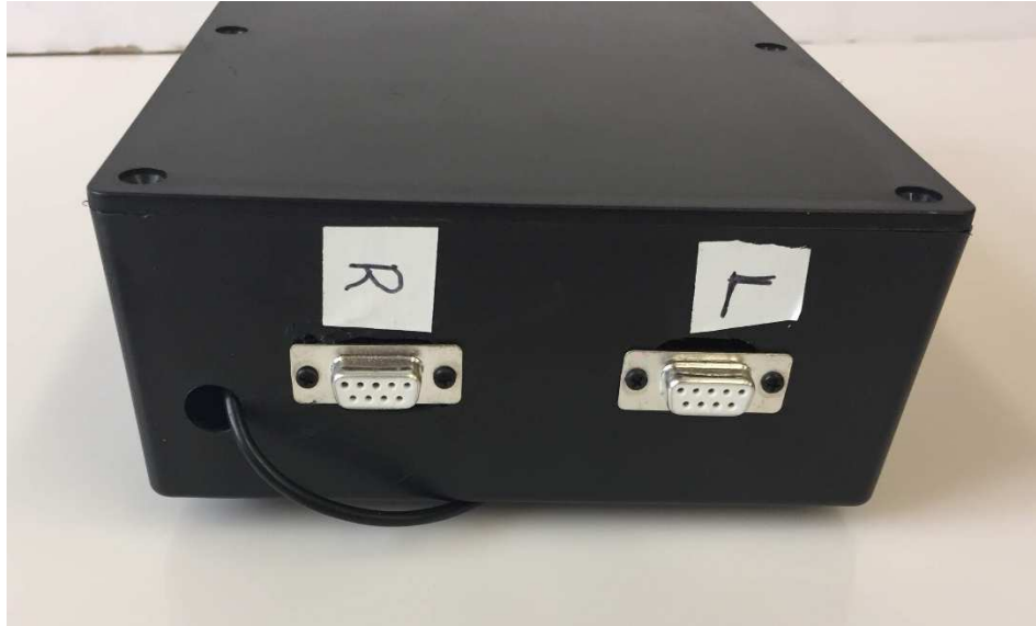
Figure 6.14: 2 DB9 connectors are used to connect the servos with the servo driver
