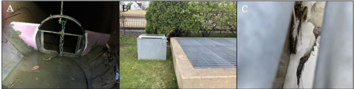
Figure 6. (A) Sampling set-up in I-35-KAc-A with adjusted weir, (B) ISCO sampling unit box used to collect stormwater from the sedimentation basin, I-35-KAc-B site, and (C) frozen stormwater in the basin during February-March, 2021
