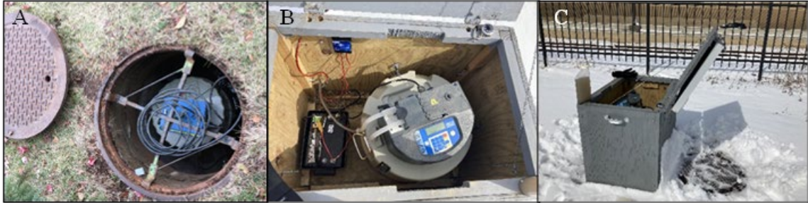
Figure 5. (A) In-manhole ISCO sampling at CE-NaCl and (B and C) Box set-up at I-35-KAc-A
