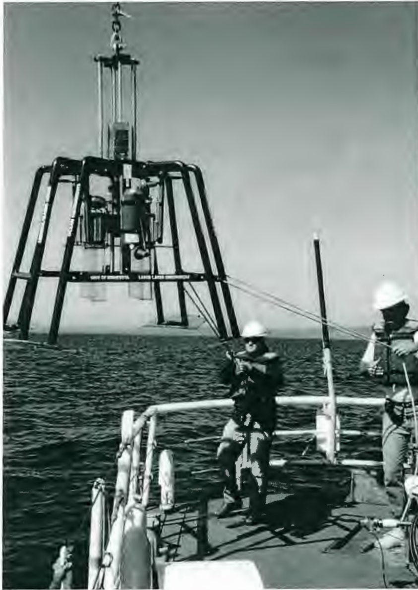
Figure 4. Ocean Instruments Multicorer being lowered overboard.
