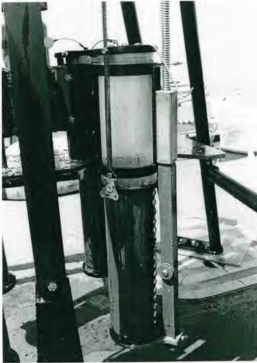
Figure 5. Multicorer tube with sediment.
