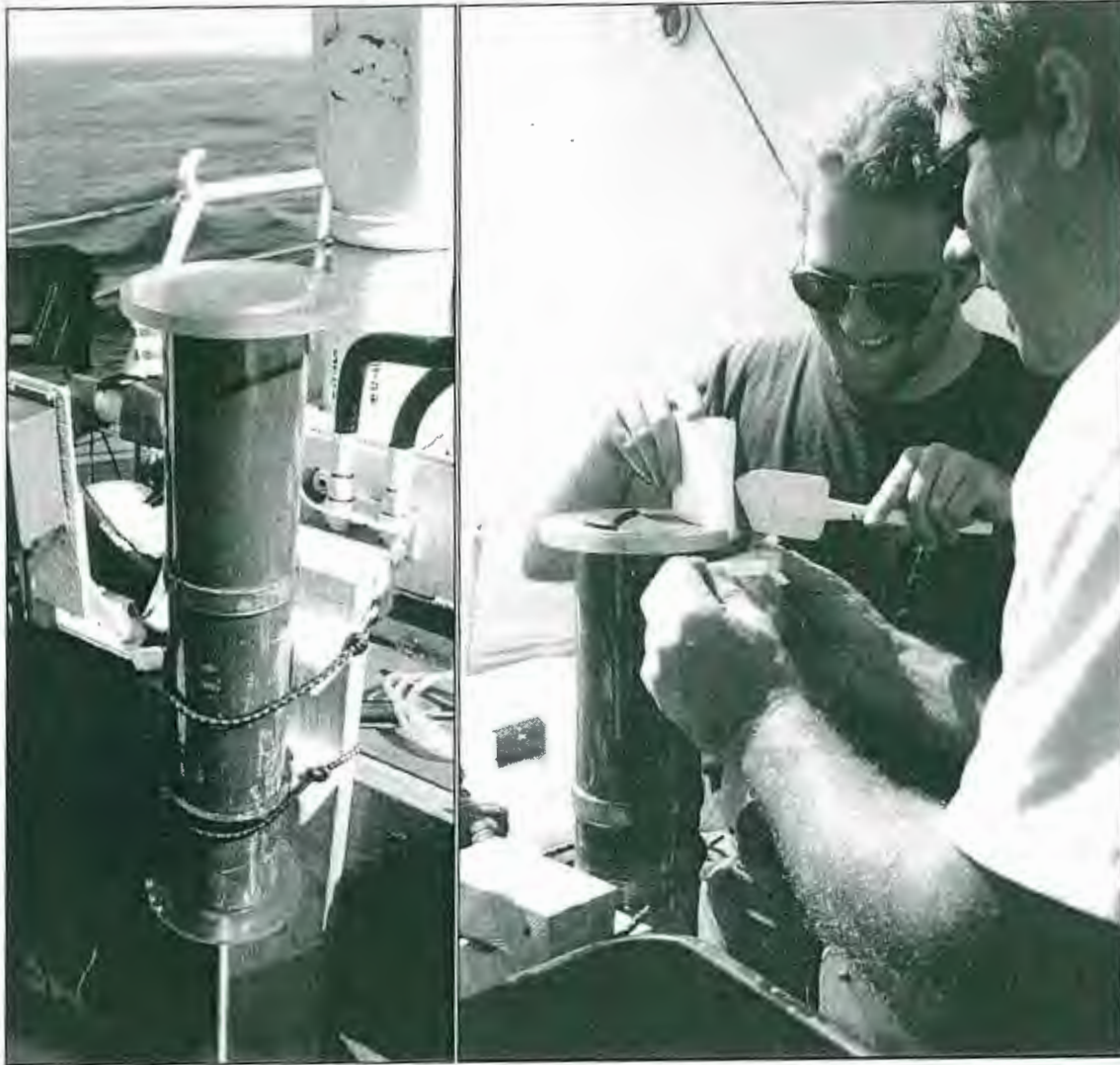
Figure 8. Extrusion process: Sediment flush with top, then raised and scraped into a bag.
