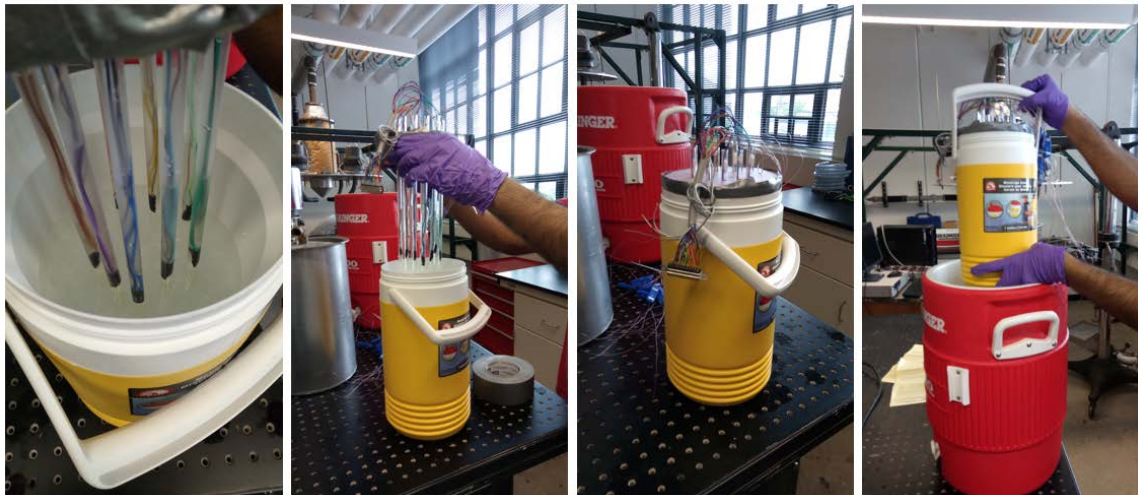
Fig. A.7 Pictures showing the arrangement of thermocouples junctions inside the reference ice bath and the corresponding wire connections.
