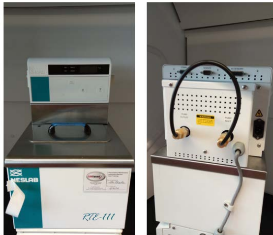
Fig. A.5 Pictures showing the front and back view of the Neslab RTE-111 chiller/heater recirculator
