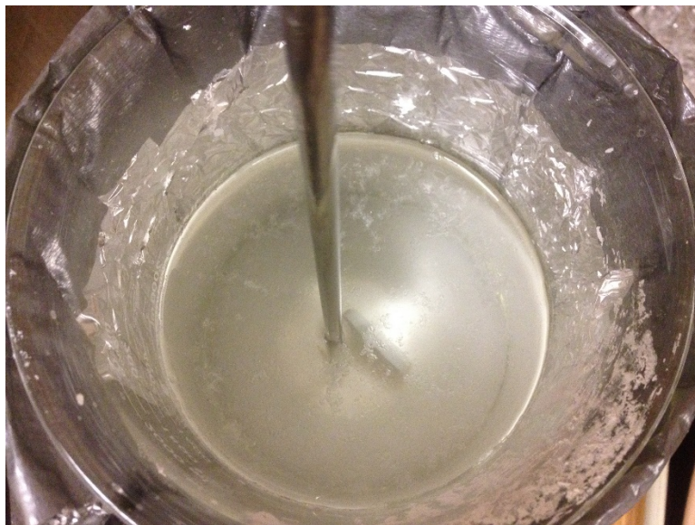
Fig. A.3 A picture of the hydration point cell as seen from the top, featuring a magnetic bead, Model 162CE SPRT, and the thermal insulation pack (around the beaker).
