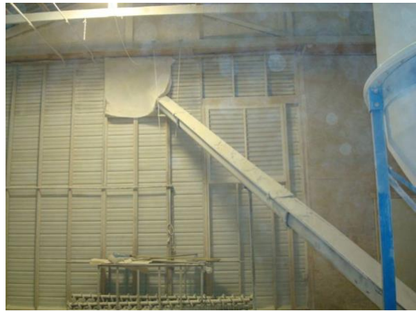
Figure 17. Auger that moves dry eggshells from a storage silo to the truck.
