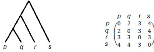
Figure 3.4: Classification tree and its corresponding distance matrix D . The distance d_{qr} is 3 meaning that there are 3 edges in the path connecting the leaf nodes q and r
