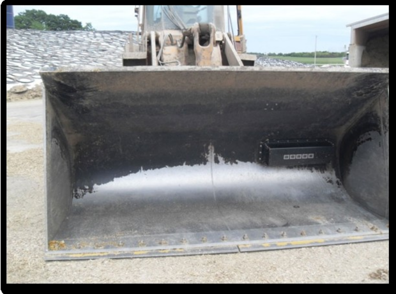
Figure 1. Bucket-mounted near infrared reflectance spectroscopy used to scan individual wet ingredients (corn silage, alfalfa silage, and high moisture corn) on real time (during ingredient addition prior to feeding) and adjust ingredient dry matter amount for each bucket load.
