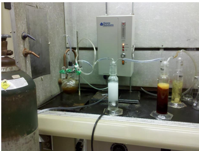
Figure 7.2. Ozone oxidation of lignin, in round-bottom flask at left and subsequent reduction of ozone released into the environment by saturation of \text{Na}_2\text{S}_2\text{O}_3 solution. Photo credit Harris, 2011.
