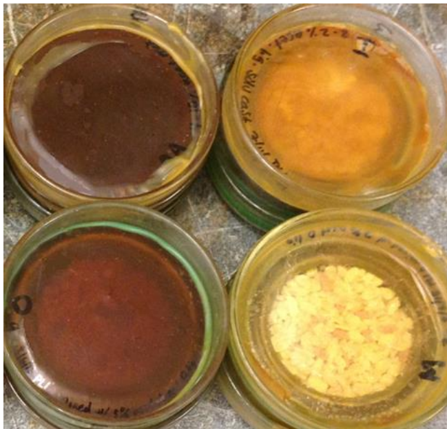
Figure 7.6. Assembled test cups with films sealed over the desiccant before being placed in varied hygrostatic conditions. Variation in color due to lignin content is apparent. Photo credit Harris, 2014.
