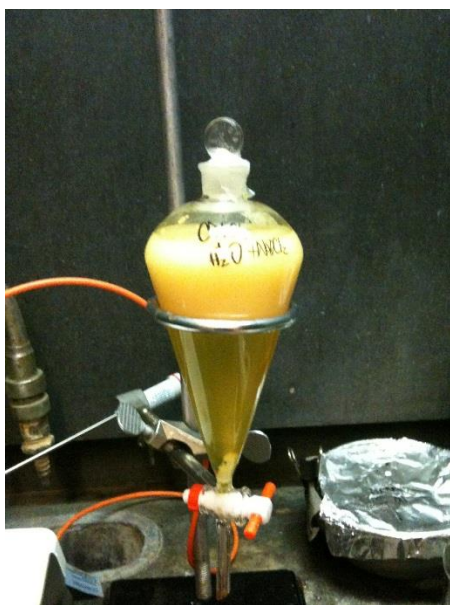
Figure 7.3. Organic and aqueous layers after peroxide treatment shown in separatory funnel. Photo credit Harris, 2016.
