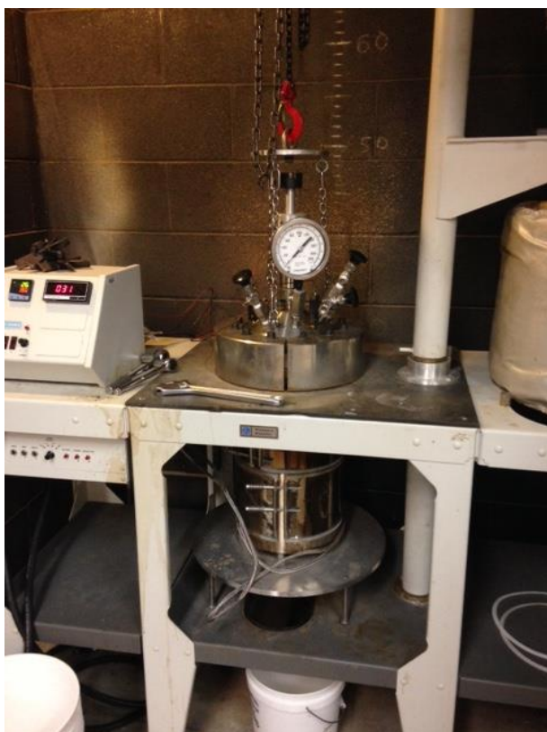
Figure 7.1. PARR 4843 pressure reactor used for organosolv method lignin extraction.
