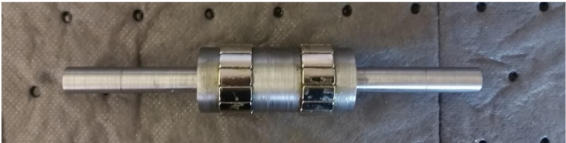
Figure 28: Shaft with N50 magnets adhered
