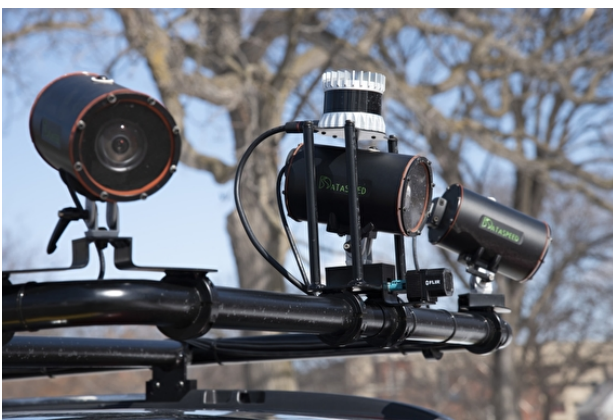
Cameras and sensors on the roof rack of the MnCAV vehicle
