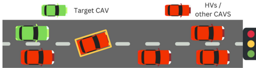
Figure 1.1: Problem description: other vehicles perform lane-changing in front of target CAV, which is inconsistent with the predicted driving plan
