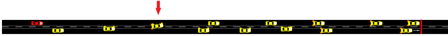
Figure 6.1: A section of the scenario, modeled traffic stream are loaded on the network, and the red vehicle is the target CAV controlled by the optimal strategy
