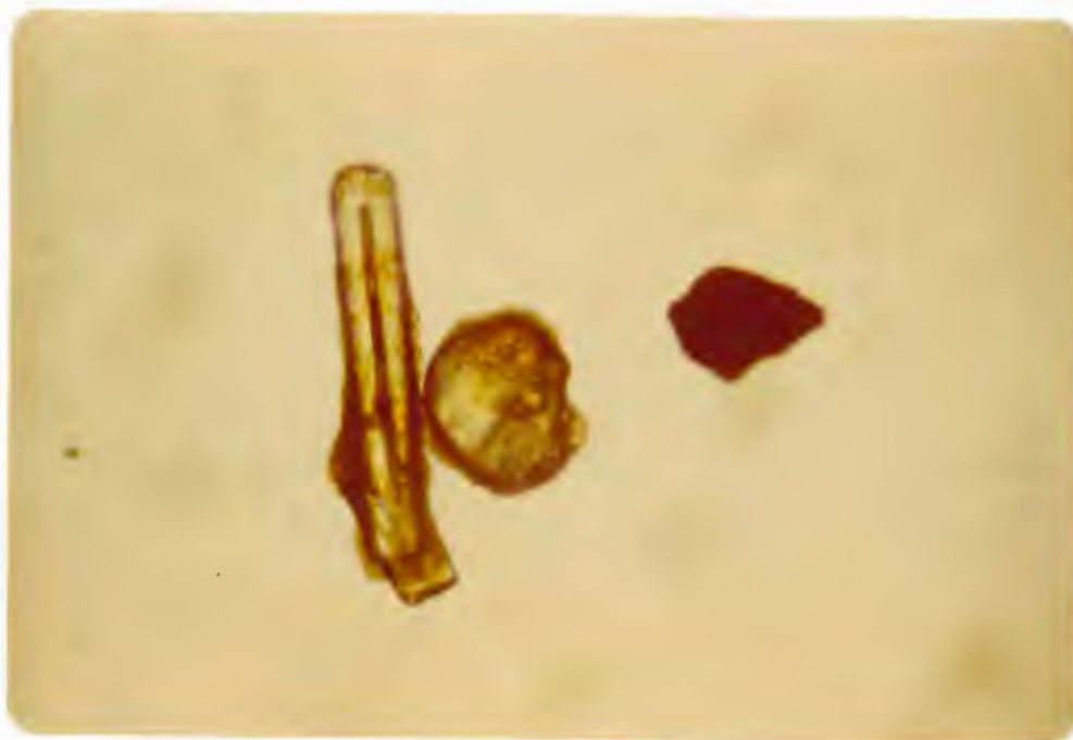
Figure 22-- Photomicrograph of two zircon grains, one with inclusion. Field of view is 1.0 mm. in width, uncrossed nicols.
