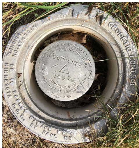
Figure 3.3 SCHREIBER geodetic marker north of the University of Minnesota.
