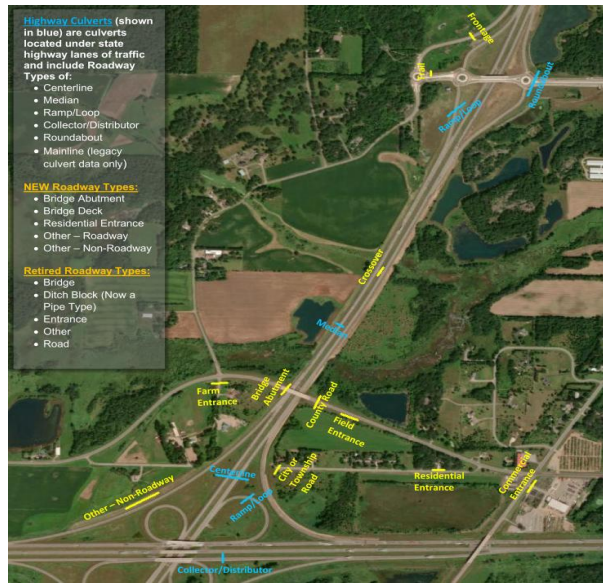
8 (b) - Description of roadway types from
