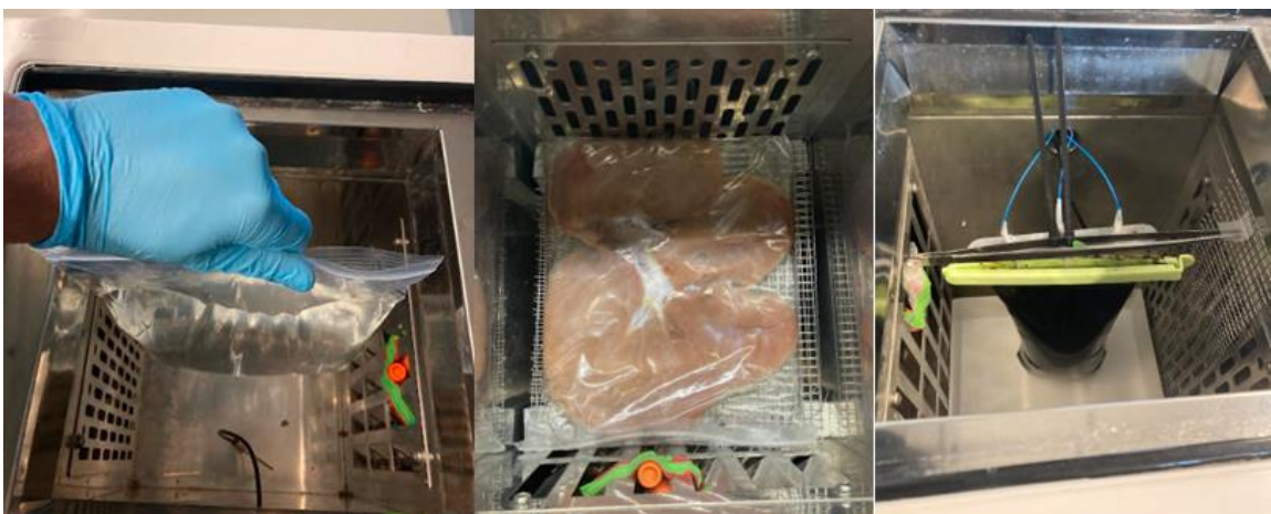
Figure S5.7: Placement of same sample volume i.e. 1L in 3 different orientations inside CRF resulting in three unique characteristics length A. L_c \sim 1.8\text{cm} , B. L_c = 1\text{cm} , C. L_c \sim 1.5\text{cm}
