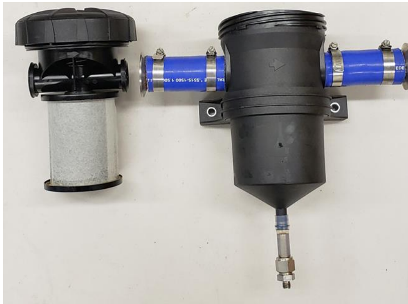
Figure 1: Crankcase ventilator assembly. Left to right: coalescing filter attached to lid, housing assembly with silicone tube inlet and outlets
