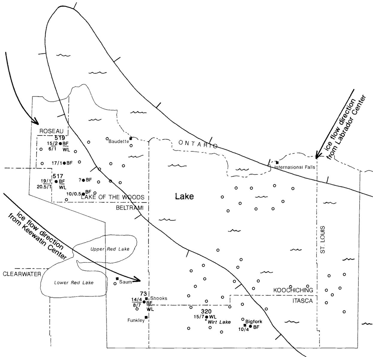
**Figure 11.** Sites where the Wirt Lake (WL) and Bigfork (BF) tills were cored. The left-hand number is average percent Paleozoic carbonate, and the adjacent number is average percent Cretaceous content of the 1-2-mm sand fraction. Also shown are the speculative flow directions and maximum extent of ice from the Keewatin center during deposition of both tills, with a proglacial lake and possible margin of ice from the Labrador center. (T = trace amount, ? = no data)
