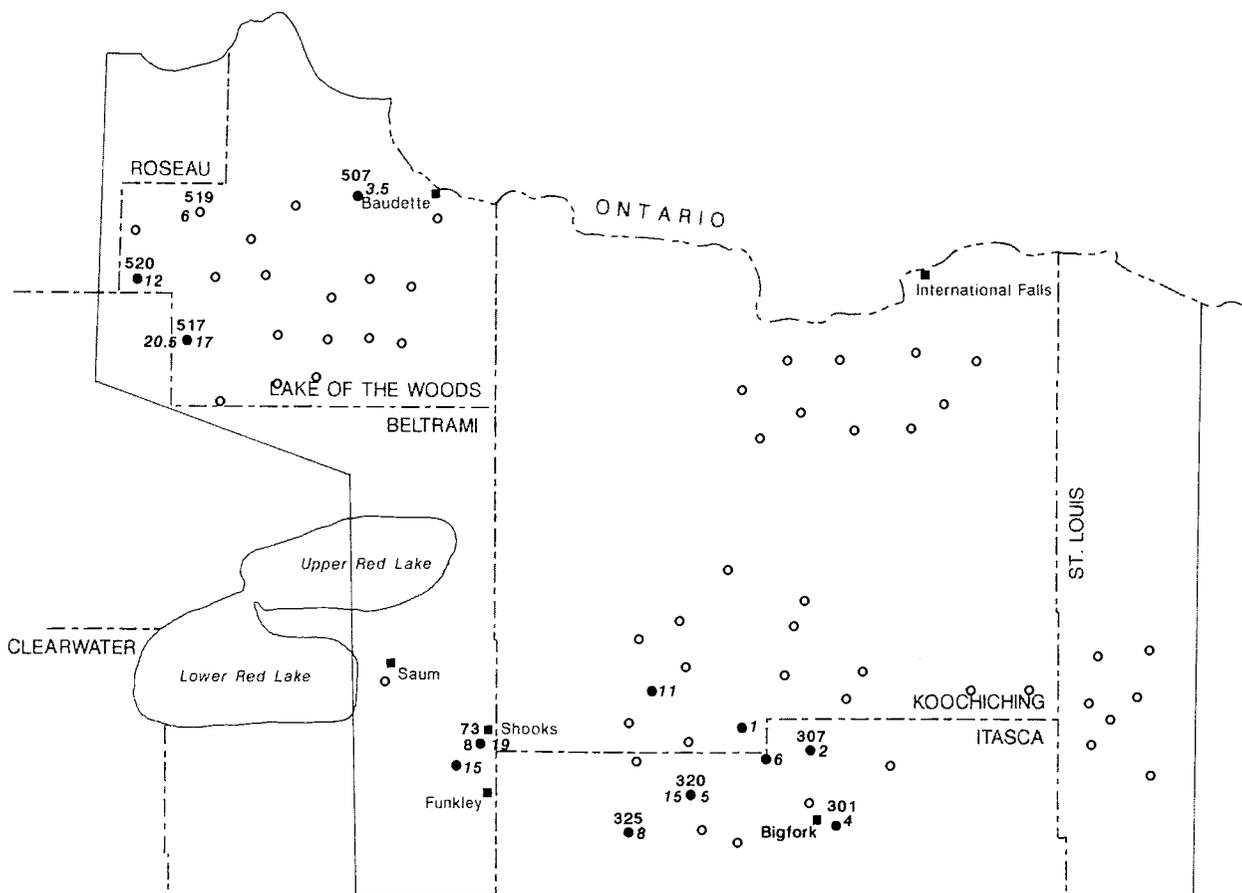
**Figure 13.** Sites where Shooks till was cored. Number on the right is average percent of Paleozoic carbonate content of the 1-2-mm sand fraction. At four sites—73, 320, 517, and 519—the number on the left is average Paleozoic carbonate of the underlying Wirt Lake till.
