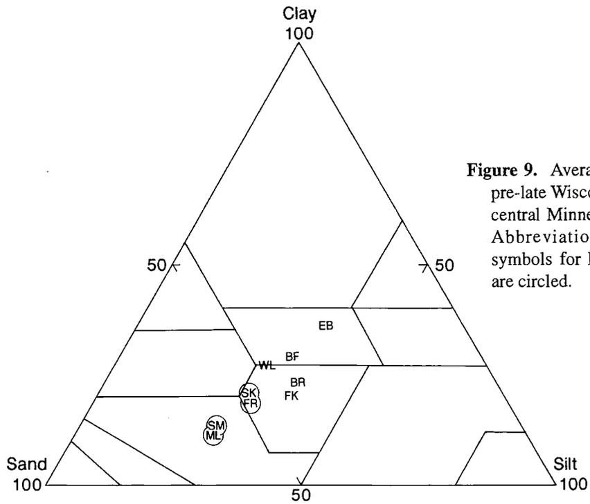
**Figure 9.** Average matrix texture of pre-late Wisconsin till of north-central Minnesota (from Table 1). Abbreviations as in Figure 6; symbols for Labrador-source tills are circled.
