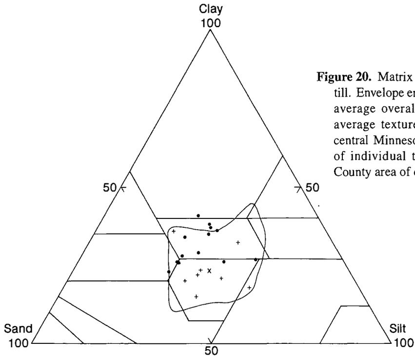
**Figure 20.** Matrix texture of the Browerville till. Envelope encloses range of values; X, average overall texture; plus symbols, average textures at each site in north-central Minnesota; solid circles, textures of individual till samples in the Todd County area of central Minnesota.
